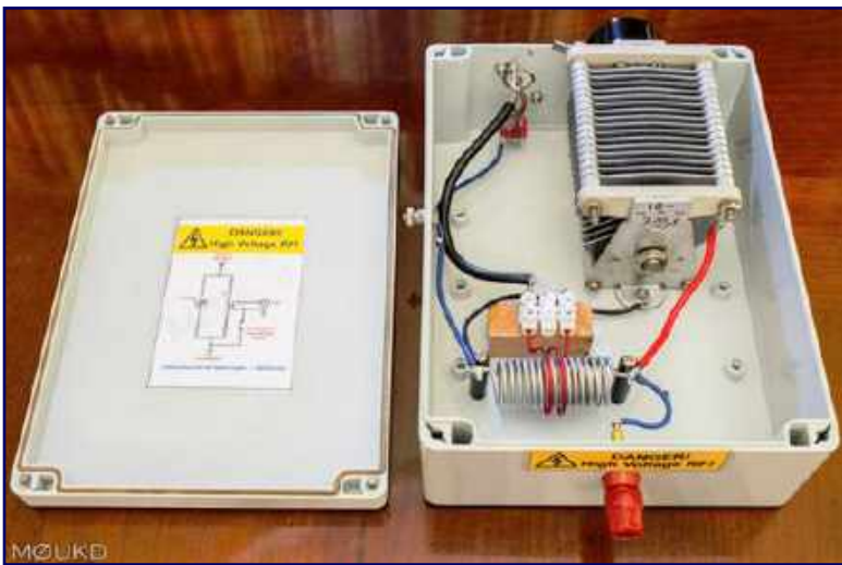
Figure 1 : M0UKD's Homebrew Transformer Matching Circuit
