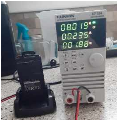
Figure 20 - Battery under 235mA discharge
