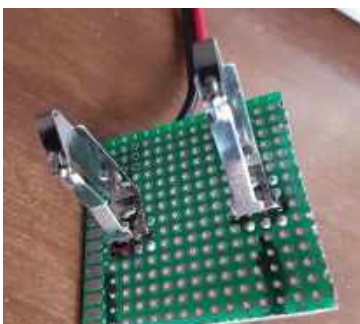
Figure 18 - Discharge cradle board
