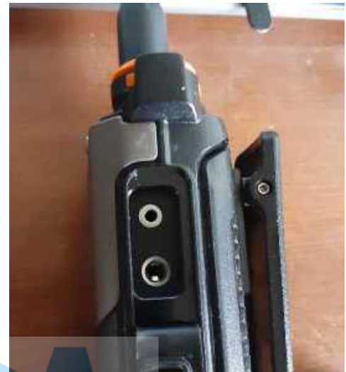
Figure 8 - Mic and speaker jacks on UV-K5(8)
