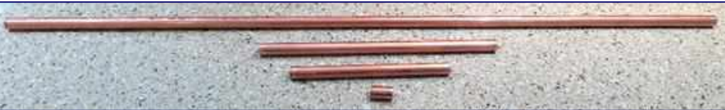
Figure 6 : Copper Pipe Cut to Length
