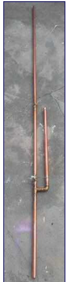
Figure 2 : 1.25M Copper Pipe J-Pole
