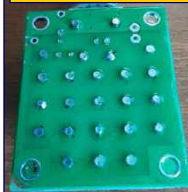
Figure 11 : PCB With Clear Polish Coating
