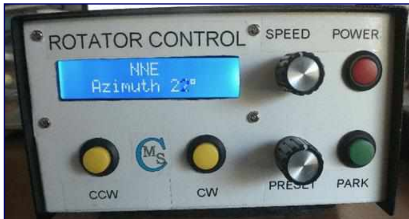
Figure 4 : Fully Operational Rotator Controller
