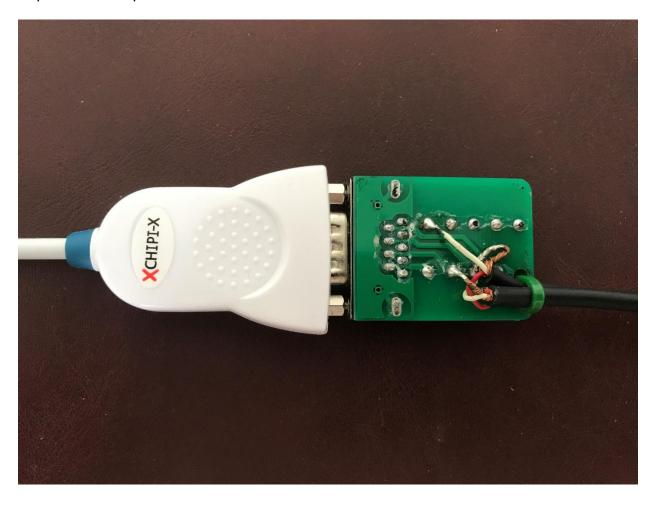
The top row of PCB terminals are DCD, RXD, TXD, RTS and GND, left to right. The bottom row of PCB terminals are RI, CTS, RTS and DSR, left to right.
