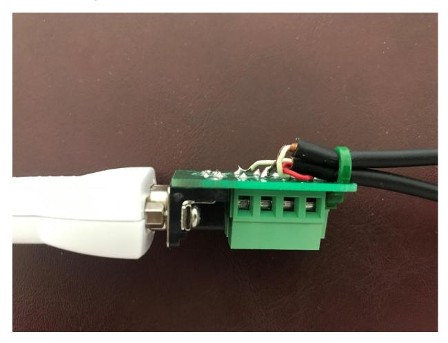
The red wire is out of the bottom cable and is connected to DSR. The white wire out of the bottom cable is connected to DCD. This is for compatibility with K3 connections. The shield is connected to RTS. This is the paddles input cable.
