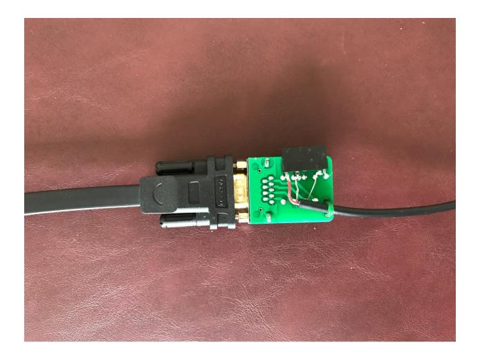
The top row of PCB terminals are DCD, RXD, TXD, RTS and GND, left to right. The bottom row of PCB terminals are RI, CTS, RTS and DSR, left to right.
