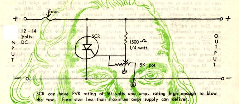
EXAMPLE: For 15 amp supply use a general electric C36F SCR. For a 25 amp supply use a GE C230F and for a 8 amp supply a GE C15F.
