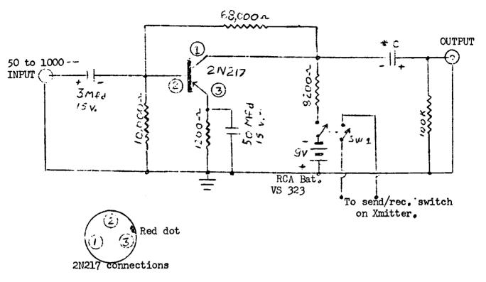
\* C may be .Ol Mfd. 400 v. paper capacitor if the "output" is coupled into a transmitter having the usual " Xtal " mike input.
