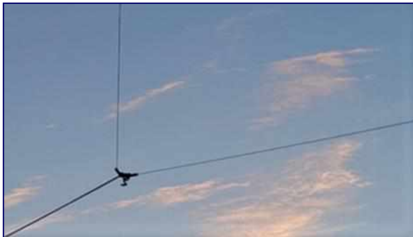
Figure 6 : Allowing the insulated wire loop to slide naturally through tubing for strain relief at tied off corners
