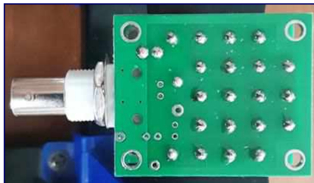
Figure 8 : All Resistors Soldered And Clipped
