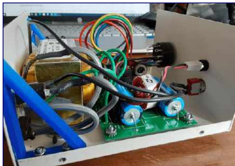
Figure 13 : Controller Side View, Showing Supports And LED Connection
