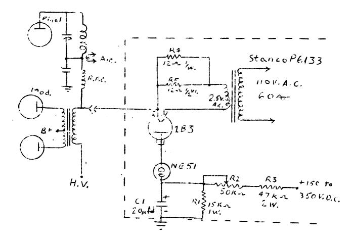
The overmodulation indicator shown above has been used in my rigs for the past six years. This circuit will work with any ham rig up to a kilowatt without any changes. The neen lamp flashes on all negative peaks of modulation of 100% or greater. That is it will glow anytime the instantaneous B to the plates of the final amplifier are at zero or in a negative direction with respect to ground.
