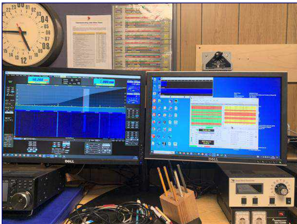
Figure 1 : The Flex SDR program and WSJT receiving meteor signals
