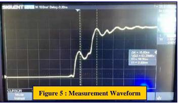
In my initial test, the  $TIME_{MEASURED}$  interval was 15.80nS. Now it is time to plug that value into the equation discussed above :
