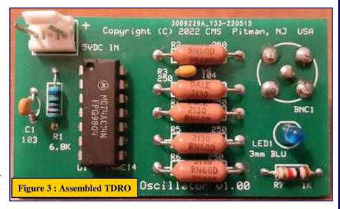
The theory behind using this oscillator to measure an unknown cable length is that the output pulse train from the oscillator is imposed upon the cable, where it travels to the opposite end of the cable. If that opposite cable end is open, the signal will be reflected back to the source. The travel time of the pulse train out and back on the cable can be measured and used to calculate the cable length.
