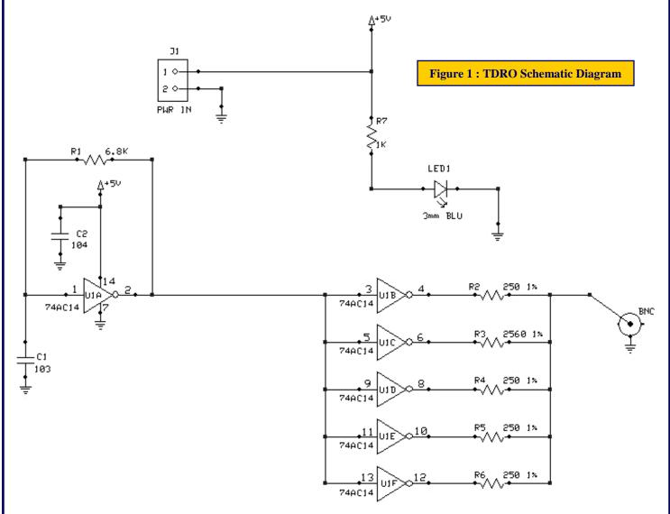
Doing some research online, I came up with a **design idea** (**Figure 1**) for a basic time delay reflectometry oscillator that is extremely simple, uses a minimal parts count, and can be tailored to the characteristic impedance of the designer's choice. In the design stages, the selection of certain components will control the oscillator output frequency. The printed circuit board layout for this circuit is shown in **Figure 2**.
