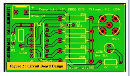
nal capacitor value of 0.00000001 farads. Upon assembly and testing, the actual oscillation frequency turned out to be 12680 hertz or 12.680kHz as stated above. Assuming that I selected an accurate constant value, the difference between the prediction and the produced frequency would likely be due to component tolerances. If I were to accurately measure and use the true component values, I could in turn calculate the actual constant value for this particular IC and power supply configuration.
