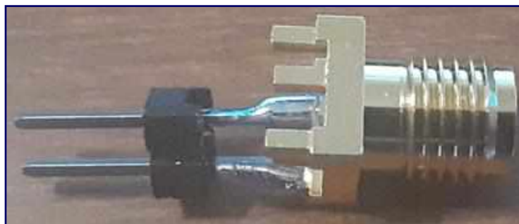
Figure 7 : RF connector adapter for NanoVNA
