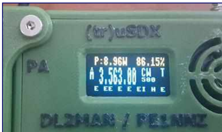
Figure 6 : Power and efficiency displayed
