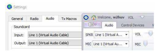
The **Line 1** Input connections appear on the **Line 1** Volume mixer on the next page as "WSJT-X v2.5.0" and "W2MMD-HF-REM, respectively. These signals appear at the WSJT-X Input **following an output volume control.**
