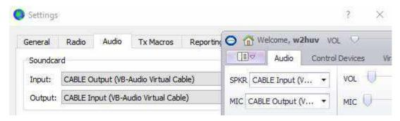
The **CABLE** Input connections appear on the **CABLE** Input Volume mixer on the next page as "WSJT-X v2.5.0" and "W2MMD-HF-REM, respectively. Note that these signals appear at the WSJT-X input.
